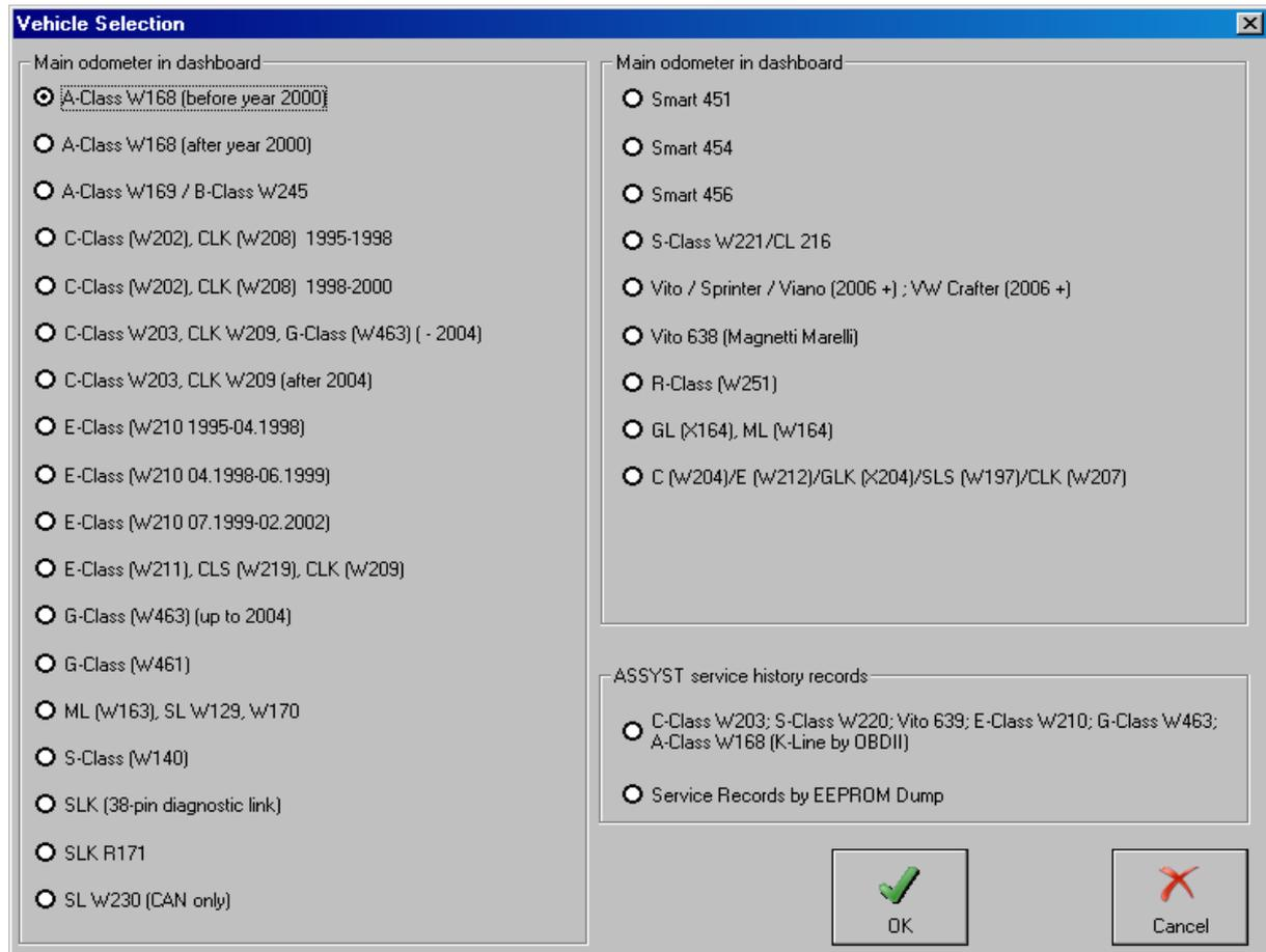
Attention: Only for W220 S-Class the odometer can not be changed by OBD ! Instead, the EEPROM of the dashboard must be read with a programmer and then the odometer should be modified by using the “Dump Tool” special function.
