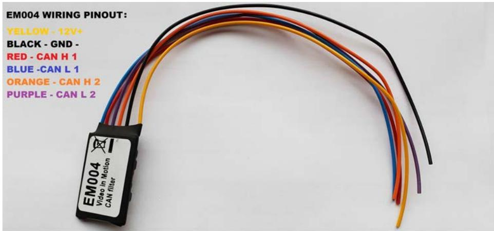
The Comfort CANBUS needs to be interrupted and the EM004 needs to be soldered to the CAN H and CAN L. You can easily tell them apart from the rest of the cables when you take the head unit out. The cables for the comfort CAN are **BROWN/ RED** and **SOLID BROWN**
