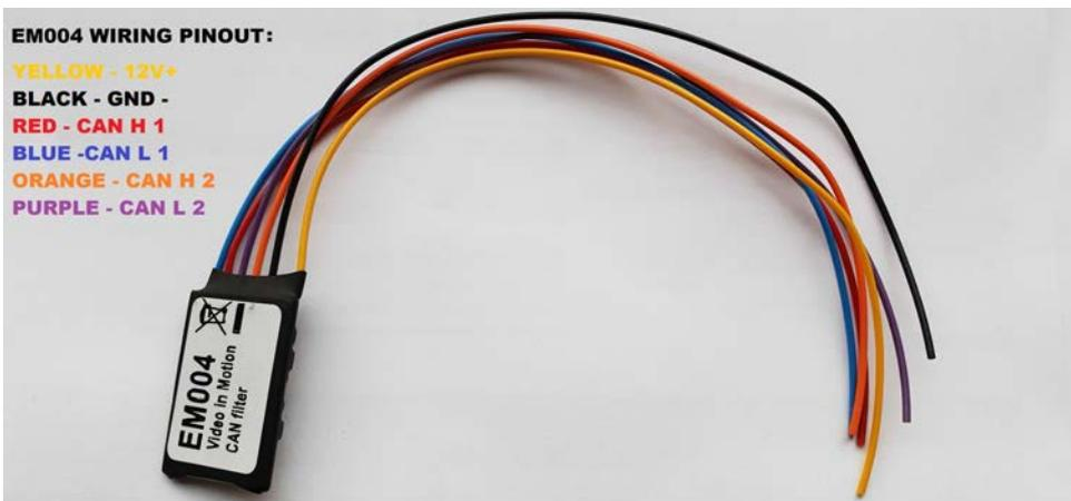
The Comfort CANBUS needs to be interrupted and the EM004 needs to be soldered to the CAN H and CAN L. You can easily tell them apart from the rest of the cables when you take the head unit out. The cables for the comfort CAN are **Yellow/ White for CAN H** and **Solid Yellow for CAN L**
