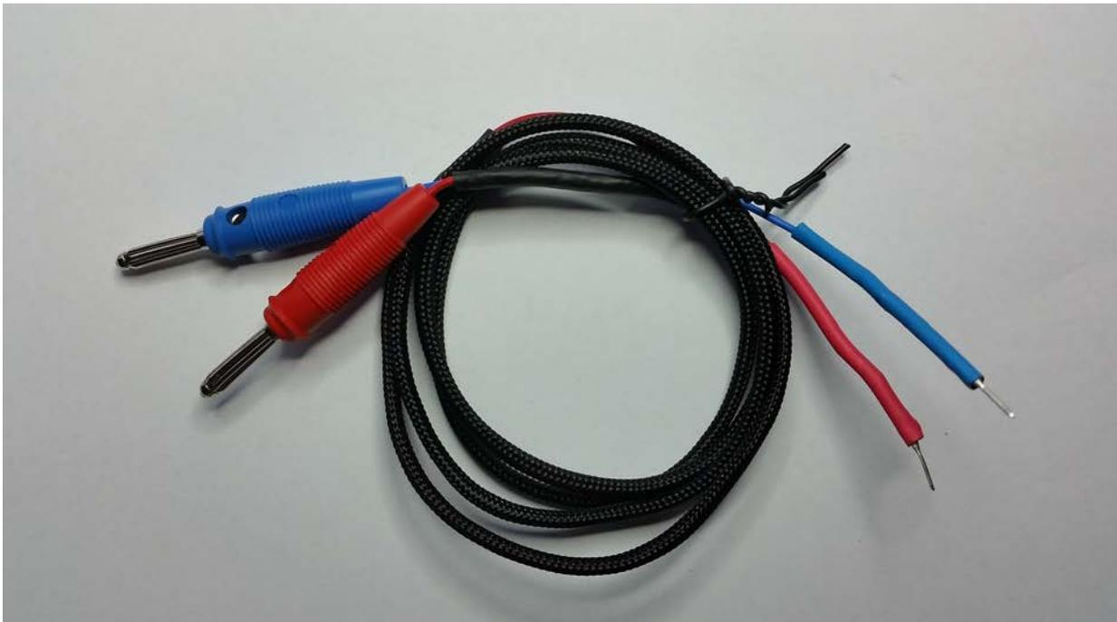
5. Abrites LIN Connector. To be used together with the main cable to connect the K- line to PIN 7 of the OBD as per the DAS manager instructions.
