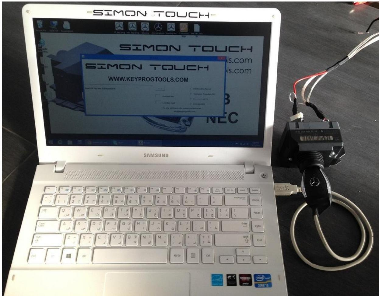
2 - Click on READ (DEVICE WILL WRITE INSERT IR TOOL IN TO EIS)
