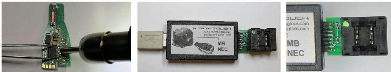
**5 - First plug the USB cable in your pc then plug the MB NEC device**
